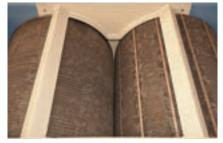
Hard face welded standard rolls for crushing hollow glass cullet. One roll is additionally cross welded for a better feeding of the input material.
